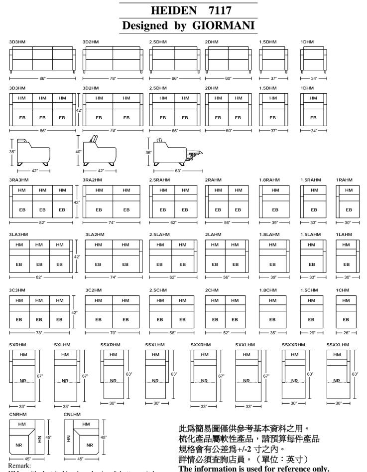
HM = with electrical head mechanism & button switch
